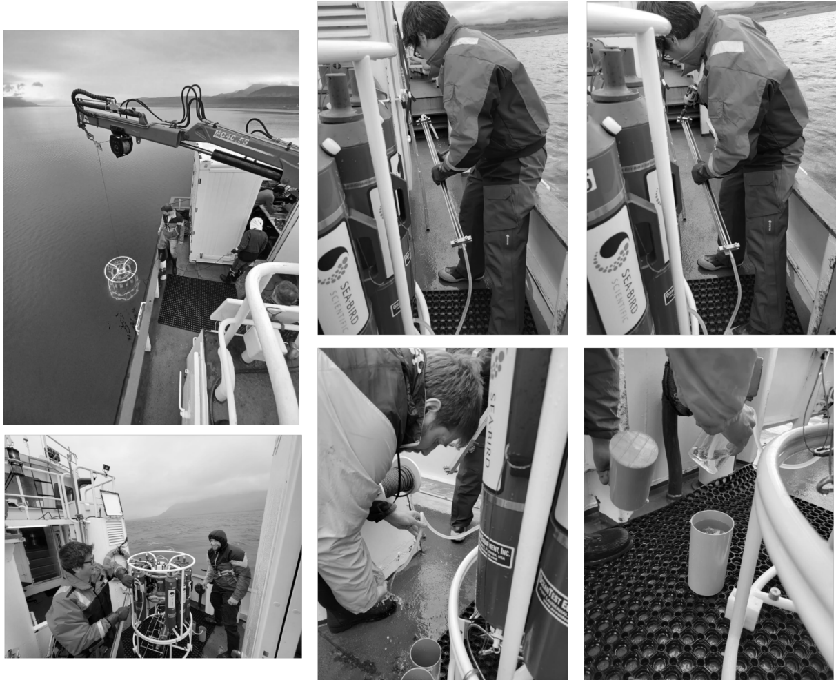
Figure 3: Selection of images showing the deployment of the CTD rosette and sampling for the two tracers from the Niskin bottles.
